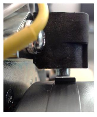
.. and that its impulse protrusions run at sensor level. (There can be problems with regenerated crankshafts.)
