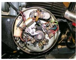
Disconnect all cables running from your old dynamo system and remove the system.
