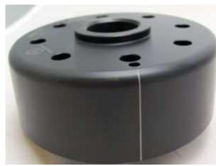
Have a look at the new rotor. You will find on its circumference a small pressed-in line. This is an ignition marking too. It is durable, but not well visible, so better highlighten it with some marker pen.
