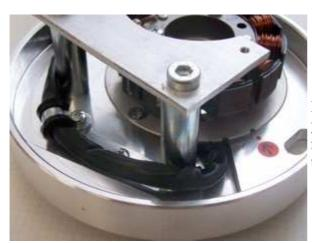
Place the holder plate for the cover, which you had taken off at the start, back. The plate rests on the 2 spacer tubes and is fixed with the 2 screws M8x60 on the base.
