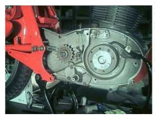
Fasten the new rotor by screwing it down with a ???. Make sure not to change the crank position. Put the spark plug in again.
