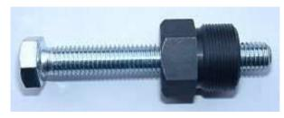
To pull the new rotor again, you need a puller M27x1,25 (part-no.: 99 99 799 00 -Not provided!-).
