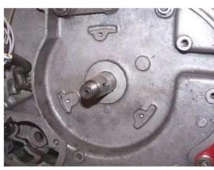
Unscrew the stator plate (3 screws) and take it off.
