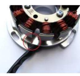
Have a look at the new stator unit. You will find at its base plate a small red marking. This is a timing mark.
