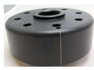
Have a look at the new rotor. On its circumference you will find a small pressed in marking. The marking is durable, but not well visible, especially when the rotor is fixed. So it is a good idea to highlighten the marking with some colour (simplest with a marker-pen).
