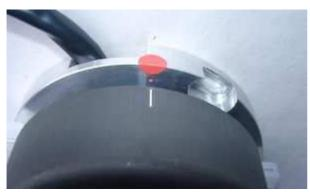
Once TDC has been found, carefully disengage the rotor again without moving the crank shaft's position from TDC. Than place it in such a way back, that the marking on the rotor aligns with the marking on the base.
