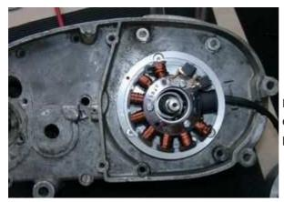
Place the preassembled unit (adapter/stator) onto the engine. Screw it down with the three provided M5 screws.
