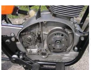
Fasten the new rotor by screwing it down. Make sure not to change the crank position. Put the spark plug in again.
