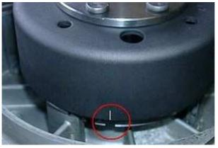
Once TDC has been found, carefully disengage the rotor again without moving the crank shafts position from TDC. Than place it in such a way back, that the marking on the rotor aligns with the **red marking** on the base, as shown in one of the pictures above.
