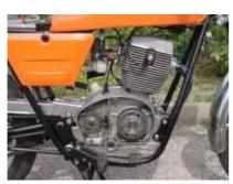
Magnet based generator with integrated ignition. Replaces complete original 6 volts magneto, inluding advance unit (govenor) points and ignition coil. Output at 12V/100W DC. Solid state ignition with own power supply from within the system and electronic advance unit giving the same advance characteristics as the original system.
