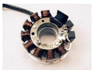
Have a look at the new stator unit. There, just after the first coppery coil clockwise after the black ones you will find a small red marking on the baseplate.
