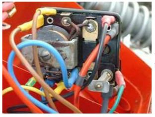
You need to deactivate the old rectifier box by shortcircuiting it with wires.
