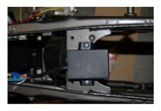
Before installing the advance unit, have a look at the small switches at the advance unit. They activate different characteristics. There are 4 switches activating different advance curves. The following gives the possible settings for the CB175:
