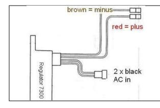
The new regulator/rectifier has 4 wires
