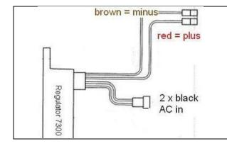
The new regulator/rectifier has 4 wires
