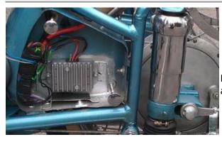
Fasten the regulator/rectifier unit, the relay and the ignition coil on a convenient place.
