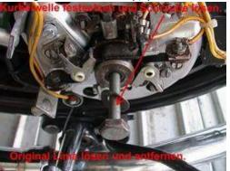
Disconnect the cables from your old generator and remove it. Unscrew the old stator and take it off the engine. Pull the rotor off, you will need a puller screw for this. Take the woodruff key from the crank. You will not need it any more. Please do not forget to do so, otherwise you will have trouble later on the assembly. (Remark: This woodruff key does not actually hold your rotor on the shaft, this is done by the
