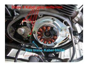
Place the preassembled base plate (with the stator) at the engine housing. Screw it tight with the 3 M6 screws and washers. The big black coil should show approximately at one o'clock. You should set the screws in the center of mounting holes, so you have the possibility for correction.
