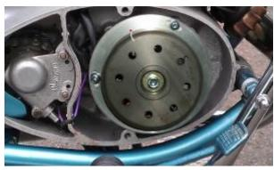
Take the rotor carefully off again without changing the crank's position. Reset it onto the crank in such a way that the marking are in line (reverse clockwise). If there is any change in the crank's position, you have to start again. In that position fasten the rotor carefully with the M8x30 nut (Please don't forget to use the washer).
