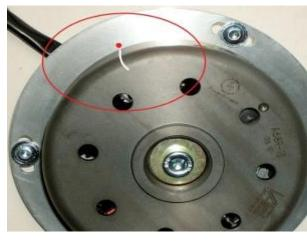
Have a look at the base plate. You find there some marking. This is also an ignition marking. At the moment of ignition both markings align as shown here in the picture.
