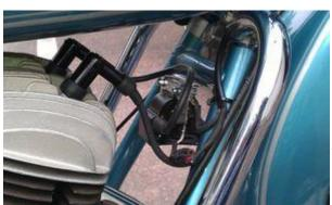
Fasten the new electronic double ignition coil on a convenient place, maybe on the frame under the tank. A clamp is in the standard accessory.
