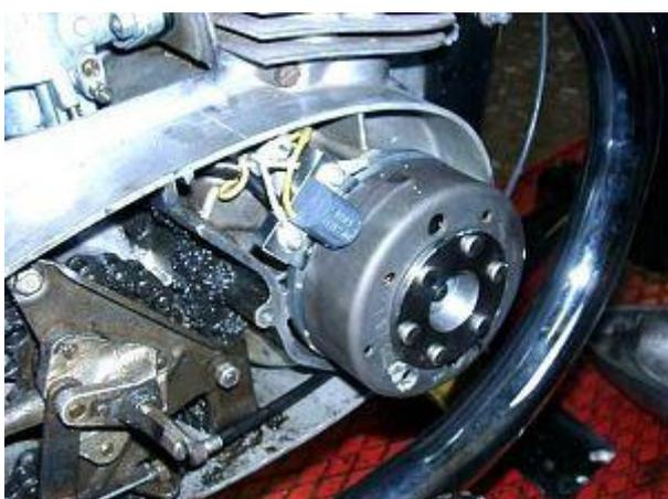
Place the rotor drum onto the crankshaft, taking care to fit the slot onto the roller pin of the crank. Check that the rotor sits well on the shaft. It happens that a roller pin is a little too high and prevents good fitment. In that case take a little material of the roller.
