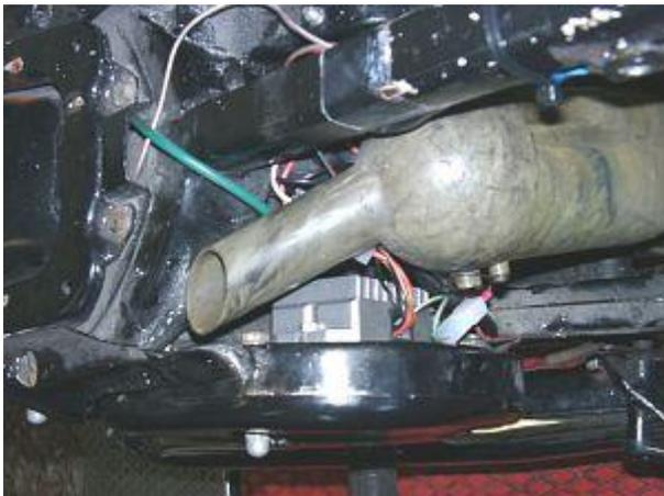
Mount the regulator/ rectifier unit of your MZ-B-Tronics at a convenient place (say [on the inner outside of the tool box](#)).
