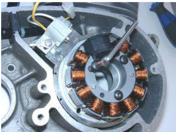
Put the stator coil back onto the plate, take care not to damage the wires.
