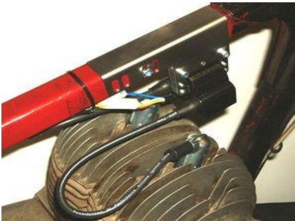
Fasten the new ignition coil at the place the old coils have been. We provide some holder with screws that should enable you to fit the coil there. To use this, fit the coil with its HT exits facing backwards (towards the seat). Unfortunately the stock coil fastening hole in the frame seems to have been drilled at random, so our holder will not always fit without modification, even though we have provided oblong holes.
