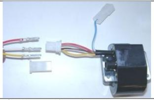
Look for the ignition coil with its female plug and the three wires (red, yellow and brown).
