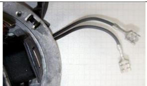
The 2 black wires running from the stator coil carry the voltage for lights, horn, flashers etc.
