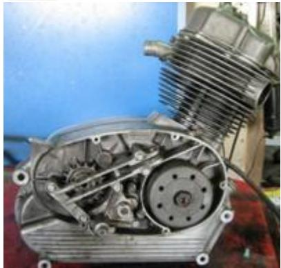
**Advantage over original system:****Generator/electronic ignition for Moto Guzzi Stornello (built after 1971) with stock magneto system**
