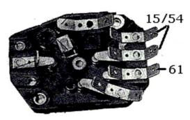
Open the headlamp housing and identify pin 61 of the main switch. Pull the red/green wire that goes to the charge control/indicator control from pin 61 and reconnect it to pin 15 or 54 instead. Should there not be a free terminal use a piggyback terminal to connect it to one of the wires there.
