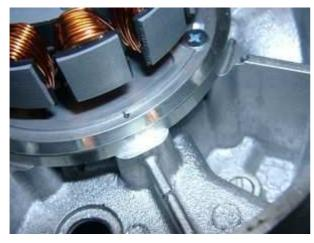
Under no circumstances effect mechanical changes on your engine casing in order to fit the system (save for pulling or breaking the pin at the stator base). Do not try to assemble the new stator without the steel ring, even if you think temporarily that fitment may only be achieved that way.
