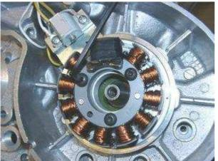
Put the stator coil back onto the plate, take care not the damage the wires. The stator has to snap in rather sharply. If it sets soft, you have probably squeezed a wire underneath!
