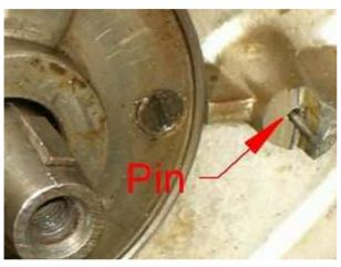
Should the arresting pin on the top right corner of the generator seat still be in place, please take it off (pull oder cut it). It will otherwise present the new system from beeing installed.
