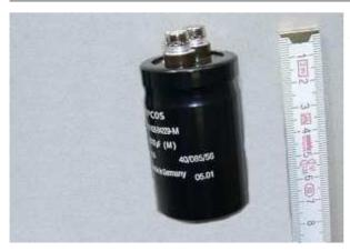
**Note:** When you make use of the <u>non-battery options</u> and have side indicators (flashers) at the same time, you will need to install a high <u>capacity</u> <u>condenser (22.000 $\mu$ F)</u> in place of the battery to smoothen the pulsing voltage. Otherwise your flasher unit will go heywire.
