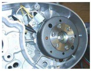
Place the rotor drum onto the crankshaft, taking care to fit the slot onto the roller pin of the crank. Check that the rotor sits well on the shaft. It happens that a roller pin is a little to high and prevents good fitment. In that case take a little material of the roller.
