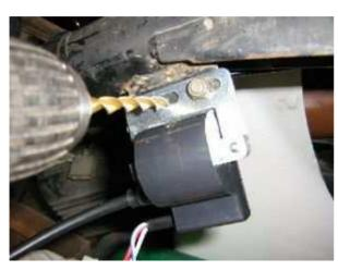
Screw the ht-cable into the ignition coil, then fasten the ignition coil on a convenient place. Secure the generator cables on the frame with the enclosed cable binders.
