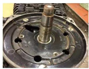
Disconnect the cables from your old magneto and remove it.
