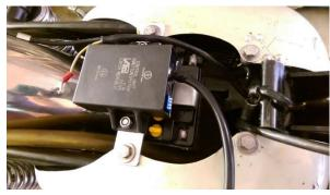
Take during the installation of the advance unit a look at the little blue switching block at the upper narrow side. There are 4 switches for choosing the different advance curves.
