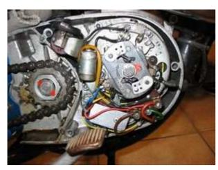
Disconnect all wires to the old dynamo, regulator and ignition coil and take those parts off.
