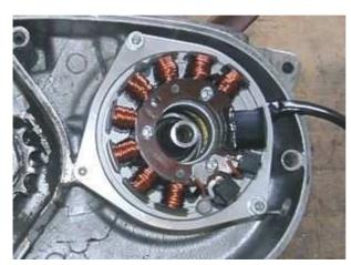
Screw down the preassembled unit (ground plate/stator), by using the original mounting holes, on the crank case with the 3 screws M6. Lead the cable carefully through the enlarged opening. Take care not to jam any wires.
