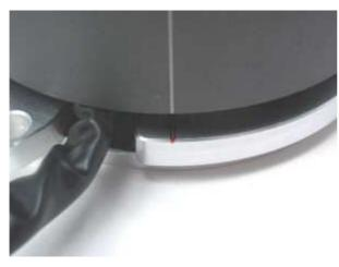
Take the rotor carefully off again without changing the crank's position. Reset it onto the crank in such a way, that the marking on the rotor aligns with the marking on the ground plate. It's very important not to change the ignition position of the crank shaft. Otherwise you have to repeat the ignition adjustment.
