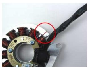
Have a look at the ground plate. You will find left of the first copper-coloured coil, left of the thick black coil, on its circumference an ignition marking.
