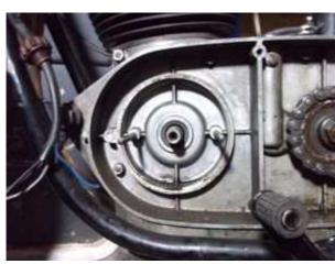
Unscrew the generator cover and take it off. Disconnect the wires from the old dynamo.
