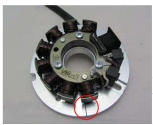
Have a look at the new stator unit. Near to the small black coils you will find a line marking on the baseplate.
