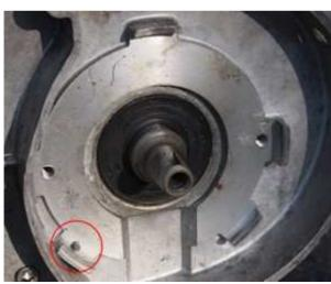
Put the base plate onto the engine in a way that this opening slots over the pin there (so there is one)
