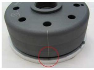
Once TDC has been found, carefully disengage the rotor again without moving the crank shafts position from TDC. Than place it in such a way back, that the marking on the rotor aligns with the marking on the base, as shown here.
