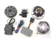
Magnet based generator with integrated ignition. Replaces complete original 6 volts dynamo, inluding advance unit (govenor) points and ignition coil. Output at 12V/100W DC. Solid state ignition with own power supply from within the system and electronic advance unit giving the same advance characteristics as the original system.
