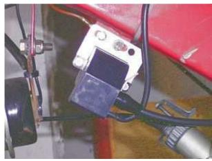
The new ignition coil should be fixed where the old coil had been.
