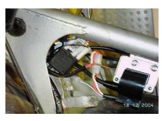
Fasten the electronic regulator on the frame.
