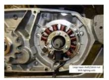
generator / electronic ignition for OSSA Phantom MX\_Rotor weight: 1000gr/35oz, rotor fastening nut with M12x1.5 LH threading AC voltage
