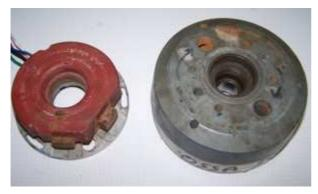
Pull the stock Motoplat rotor off, you will need a puller for this. Unscrew the old stator and take it off the engine.
