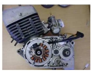
Place the preassembled unit (ground plate/stator) at the ignition system mounting of the crank case. Screw it tight with both M5 screws. You should set the screws in the center of mounting holes, so you have the possibility for correction. Please don't forget to use the washers.
