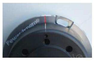
Take the rotor carefully off again without changing the crank's position. Reset it onto the crank in such a way that the marking on the rotor aligns with the marking on the stator. If there is any change in the crank's position, you have to start again. In that position fasten the rotor carefully with the M8x30 nut. (Please don't forget to use the washer!)
