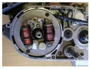
Disconnect the cables from your old generator and remove it. Unscrew the old stator and take it off the engine. Pull the rotor off, you will need a puller screw for this.
