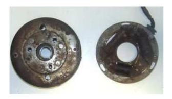
Disconnect all wires from the old generator and ignition coil and remove these parts.
