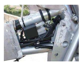
Fasten the new regulator/rectifier at a convenient place too, maybe in the frame triangle beneath the tank (screwed against the ignition coil) or beneath the seat or the side casings.
