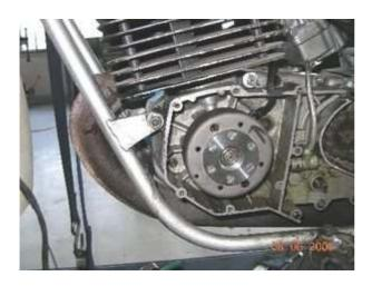
Take the rotor carefully off again without changing the crank's position and reset it onto the crank in such a way that the marking on the rotor aligns with the marking on the stator. In that position fasten the rotor carefully with the original nut.
