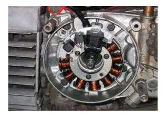
Put the new stator assembly into the place of your old generator. Fasten the plate with the 2 screws M6. Take care to not jam any wires under the plate.
