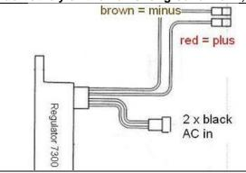
The new regulator/rectifier has 4 wires
