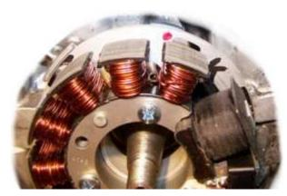
Unhopefully the ground plate's ignition marking isn't visible now. You have to either continue the marking to the motor or notice a marked point at the motor that is visible beyond the rotor.
