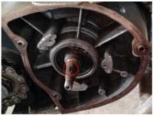
Remove the engine cover. Then remove the original generator and ignition system. These parts will not be needed with the new system but could be retained to restore the motorcycle to original condition in a future restoration.
