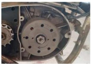
When the rotor is tightened with the stock rotor nut, replace the spark plug. If you used the rear wheel to rotate the engine, shift back to neutral.
