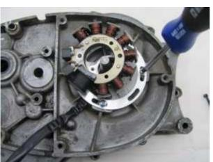
Install the base plate and the stator tower on the engine case with the three provided M4x16 screws and washers. Examine the base plate of the new stator.
