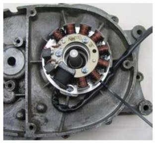
Now you have to replace the stator on the ground plate. Take care, that no cable is pinched. The coil has to be fitting good on the ground plate - nearly "hearable engage". If is it ain't so, and the coil fits "soft" on the ground plate, is a cable in the way and there is a risk of damaging by contact of the rotor.
