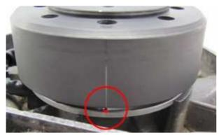
Remove the spark plug and bring the piston into ignition position. For better control when turning the engine over, shift the transmission into fourth gear and use the rear wheel to rotate the engine. Alternatively, use the new rotor to turn the engine by attaching it to the crankshaft and turning it until the piston is at top dead center.
