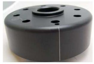
Now examine the rotor. Notice that there is a small line inscribed on the exterior of the rotor housing. This is also a timing mark. It will be used to align the rotor during installation.
