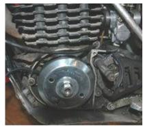
Ignition for Bultaco 250/350 with crankshaft nut M18 with rotor 2kg
