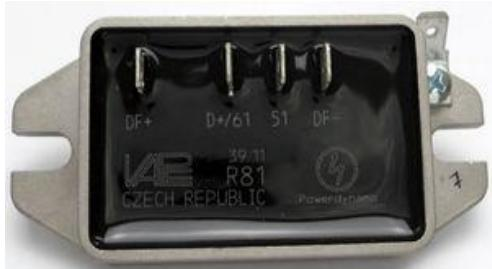
**Electronic replacement regulator for original 6-volt motorcycle dynamo systems, voltage regulating, for negative ground (minus to chassis)**
