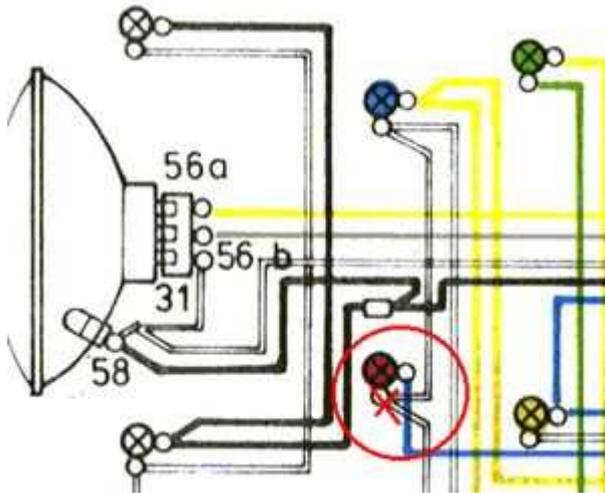
Disconnect the charge control light from ground (the red pilot light in the cockpit) and reconnect it to switched plus (pin 15 of the ignition lock). Should you want to drive without battery you need not do this change. In that case you will leave the green/red wire from the new regulator (see below) unconnected as the charge control will not light anyway due to the missing battery.
