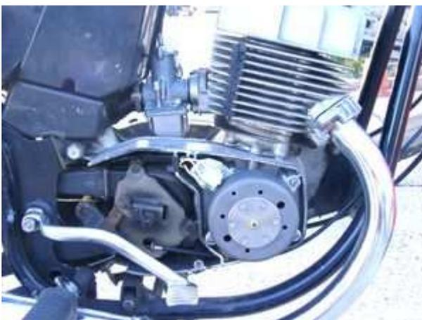
Place the new rotor onto the crankpin. Make sure that the arresting pin sits in the rotor's groove and the rotor sits tightly on the shaft. To pull the rotor again (when needed) use a simple screw M12 as a puller.
