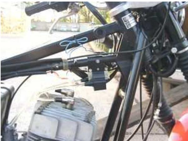
Fasten the new ignition coil with its holder at the frame under the tank. Try to put this coil as far as possible to the front (and away from the heat of the cylinders).
