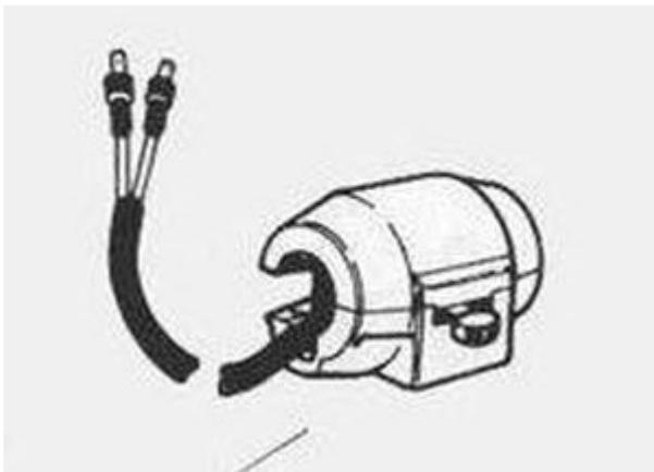
Disconnect the engine stop switch at the righthandside of the handlebar from plus and reconnect it to ground.
