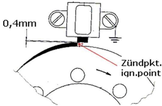
Turn the rotor slowly by hand and check clearance between the sensor and one of the rotor noses. This has to be ca. 0,4mm. You may adjust the gap by loosening the 2 holder screws of the sensor and shifting it a little.
