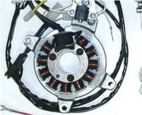
Place the premounted stator unit onto the engine. The pickup module will show towards about 11 o'clock. It will fit however only in one position, so nothing can go wrong there.
