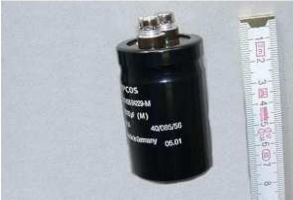
**Note:** When you make use of the [non-battery option](#), you will need to install a high [capacity condenser \(22.000µF\)](#) in place of the battery to smoothen the pulsing voltage. Otherwise your flasher unit will go heywire.
