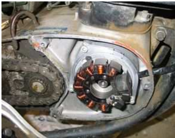
pic shows dynamo engine and stator with lighting coils
