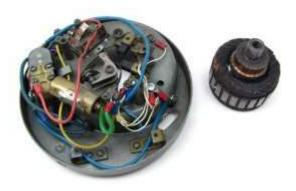
Disconnect all cables running from your old dynamo system and remove the system.
