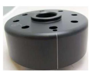
Have a look at the new rotor. You will find on its circumference a small pressed-in line. This is an ignition marking too. It is durable, but not well visible, so better highlighten it with some marker pen.
