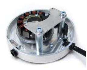
Place the holder plate for the cover, which you had taken off at the start, back. The plate rests on the 2 spacer tubes and is fixed with the 2 screws M8x60 on the base.
