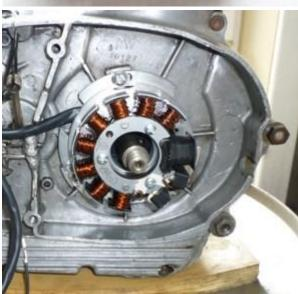
Place the pre-assembled stator assembly onto the engine, same place as your original stator had been sitting. The wire should exit like the stock system. Screw the plate down with the 3 screws M5 provided.
