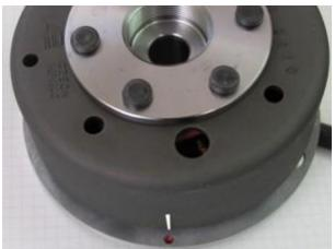
Once TDC has been found, carefully disengage the rotor again without moving the crank shaft's position from TDC.
