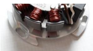
Have a look at the new stator unit. You will find a red marking at its base plate. This is a timing mark for ignition. This mark will be covered by the rotor, you should continue it on the engine housing.
