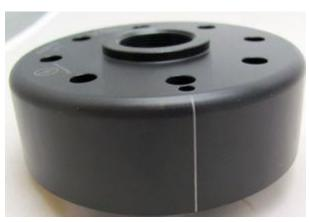
Have a look at the new rotor. On its circumference you will find a small pressed in marking. The marking is durable, but not well visible, especially when the rotor is fixed. So it is a good idea to highlighten the marking with some colour (simplest with a marker-pen).
