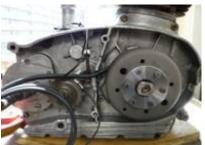
generator/electronic ignition for <u>MV Agusta 150RS</u> made in 60s (base plate diameter 110mm) NOT for later 150RS ''S'' (with base plate diameter 94mm)!
