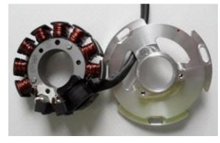
Should you take the stator coil completely off its base, make sure to reset it at the correct position. The wire has to lead through the correct opening (see picture). Otherwise you get a change in timing by 120° and the coloured markings are no longer correct.
