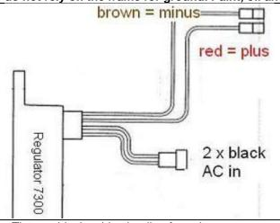
The new regulator/rectifier has 4 wires
