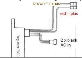
The new regulator/rectifier has 4 wires
