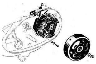
To disangage the new rotor again, you need a puller M27x1,25 (part- no.: 99 99 799 00 **-Not provided!-**).
