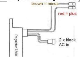
The new regulator/rectifier has 4 wires
