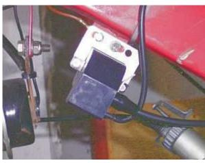
Fasten the new ignition coil at the frame (say same place, as the original). Leave one screw loose, you have to connect a ground cable here.
