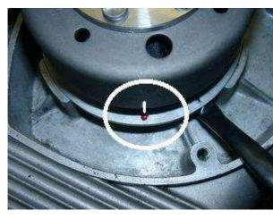
Take the spark plug out and bring the piston into top dead center position (TDC), that is the highest point the piston can reach. As this is difficult to do with the kick lever, place the new rotor onto the crankshaft (do not screw it down) and use it as a handle to turn the crank.
