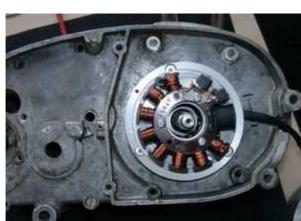
Place the new stator unit onto the engine and fasten it there with the 3 screws provided. The wire will have to show towards the wire exit.
