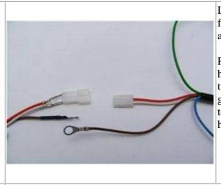
Look for the advance unit with its female plug and the two wires (red and white).
