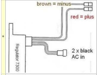
The new regulator/rectifier has 4 wires
