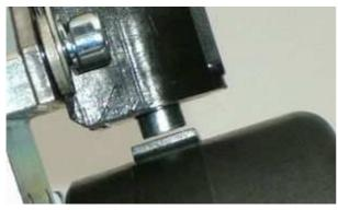
Check that the metal pin of the sensor runs about middle of the trigger sign on the rotor. The more it is outside, the harder starting is.
