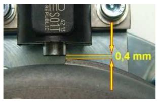
Put the rotor on but do not tighten it yet. Than turn the rotor slowly by hand and check clearance between the sensor and one of the rotor noses. This has to be ca. 0.4-0.5mm.
