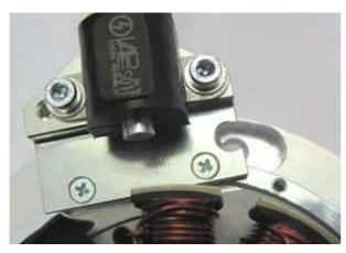
The stator assembly is fastened by 3 supplied socket head screws M6x12. As the one of them near the pickup is obscured by the pickup holder, the holder has been opened a little so that the allan key can be applied. There is no need to take the sensor (pickup) holder off.
