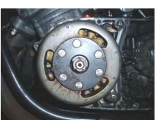
Disconnect all wires to the old magneto, points. regulator, rectifier, CDI and ignition coils and take those parts off.
