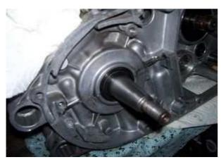
Take the woodruff key from the crank pin. It will not be needed anymore and prevent assembly. If you forget this right at start, you will have to take the whole new unit off again to get access to the key.
