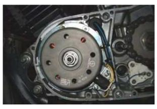
Tighten the rotor with the stock nut, not forgetting the supplied washer and bush as the threading is quite long. To undo the rotor use a puller M27x1,25. With that the work on the engine is finished. Put the spark plugs back.
