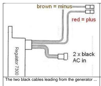
The new regulator/rectifier has 4 wires
