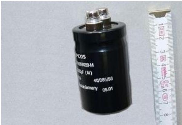
**Tip no. 1:** When you make use of the non-battery options and have side indicators (flashers) at the same time, you will need to install a high capacity condenser (22.000 $\mu$ F) in place of the battery to smoothen the pulsing voltage. Otherwise your flasher unit will go heywire.
