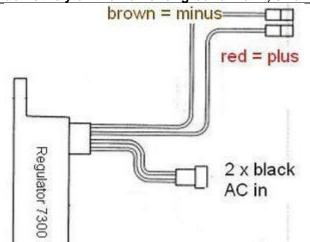
The new regulator/rectifier has 4 wires
