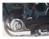
Magnet based generator with integrated solid state ignition Output at 12V/100W DC.
