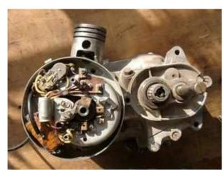
Disconnect the wires from the old dynamo and take it off. Pull the rotor of the crank.
