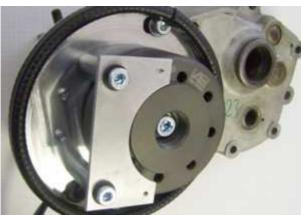
To disengage your new rotor again, you will need a puller M27x1,25 (part-no.: 99 99 799 00 -Not provided!-).
