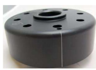
Take a look at the new rotor. You will find on its circumference a small pressed-in line, an ignition marking too. Both aligns at the point of ignition.
