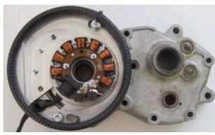
Take the preassembled cover holding plate off the new generator. Put the ground plate/stator unit onto the crank case and screw it down with the 2 screws M8. Don't forget to use the on one side cutted washers.
