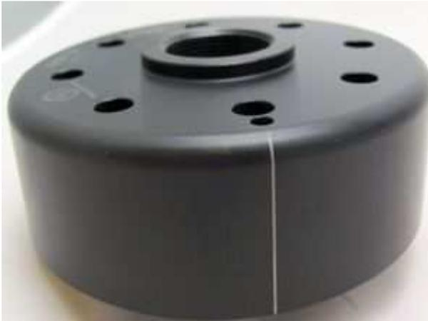
Have a look at the new rotor. You will find on its circumference a small pressed in line. That is an ignition marking. It is durable, but not well visible, so better highlighten it with some marker pen.
