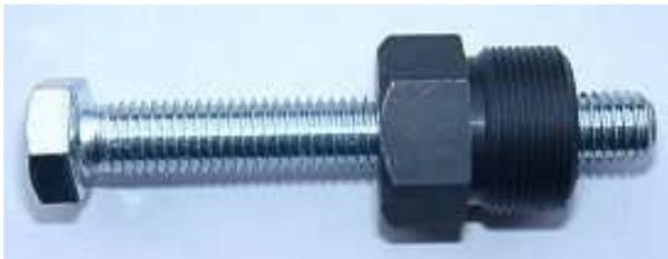
To disengage your new rotor again, please use the puller M27x1.25 (part-no.: 99 99 799 00) provided.
