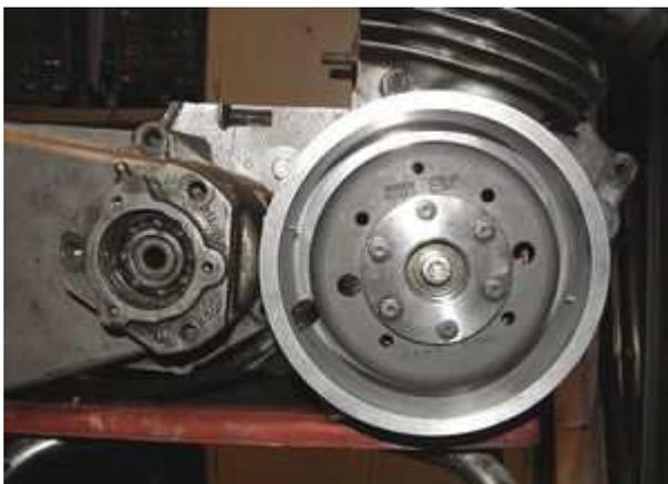
Place the rotor onto the shaft.
