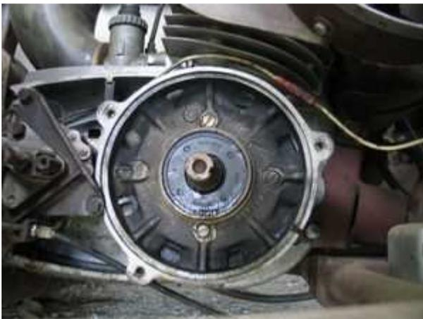
Place the stator unit onto the engine and fix it with the 3 stock clamps.
