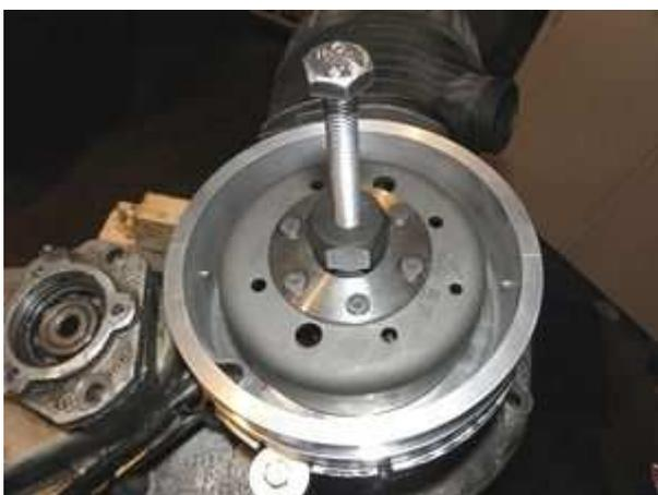
In that position, screw the rotor down with the provided screw M8x1 (place the washer there).
