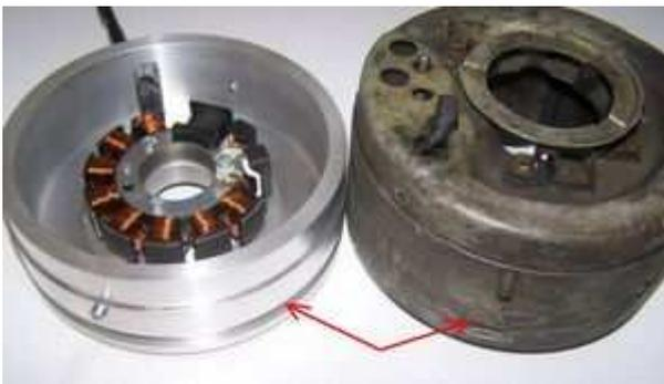
Have a look at the new stator unit. It has at the bottom some groove going all around the unit.
