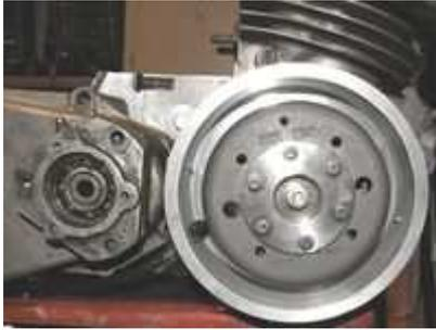
Magnet based generator with integrated ignition. Output at 12V/150W DC. Solid state ignition. Replaces old dynamo, points, ignition coils.
