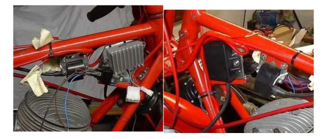
Before installing the advance unit, have a look at the small switches at the advance unit. They activate different characteristics. There are 4 switches.
