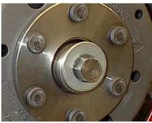
Fasten the new rotor by screwing it down with the provided screw M7.
