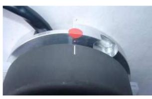
Once TDC has been found, carefully disengage the rotor again without moving the crank shafts position from TDC. Than place it in such a way back, that the marking on the rotor aligns with the **red marking** on the base, as shown in one of the pictures above.
