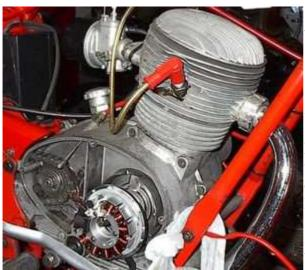
Put the base plate with the stator hanging loosely from the unit into the place of your old generator. Put the stator coil back onto the plate, take care not the damage the wires. The stator has to snap in rather sharply. If it sets soft, you have probably squeezed a wire underneath!
