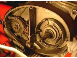
Unscrew the stator housing and take it off. Pull the rotor off, you will need a puller screw for this. Take the woodruff key from the crank. You will not need it any more. Please do not forget to do so, otherwise you will have trouble later on in the assembly. (Remark: This woodruff key does not actually hold your rotor on the shaft, this is done by the cone. It simply guides to the correct setting which will now be otherwise achieved.)
