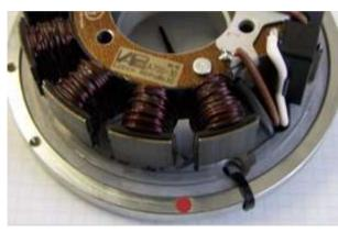
Have a look at the new stator unit. You will find near the larger black coil a small red marking on the baseplate.
