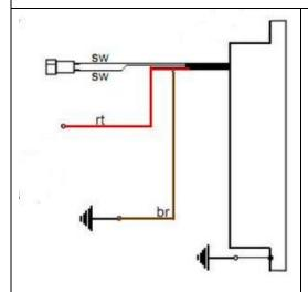
The new regulator/rectifier has 4 wires
