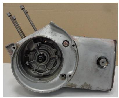
Disconnect the wires from the old dynamo. Pull all wires out of the engine housing. Take the old system off (you will need a puller for the flywheel).
