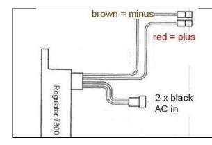
The new regulator/rectifier has 4 wires
