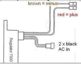
The new regulator/rectifier has 4 wires
