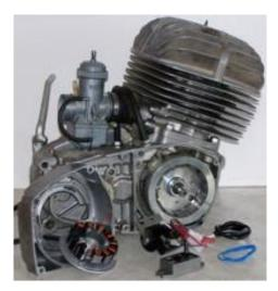
Generator/electronic ignition for: CZ 250cc moto-cross (typ 980) from Sidepipe (1968) to 1974, CZ 380cc (typ 981), early CZ 125 motocross up to 1974 and possibly (not confirmed) CZ500
