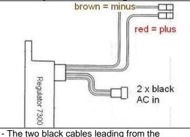
The new regulator/rectifier has 4 wires
