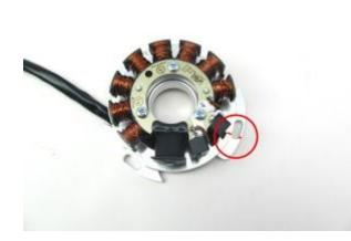
Place the pre-assembled stator unit onto the engine's magneto seat and screw it down there with the 3 screws M5.
