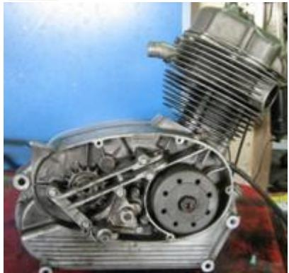
**Advantage over original system:****Generator/electronic ignition for Moto Guzzi Stornello with stock magneto system**
