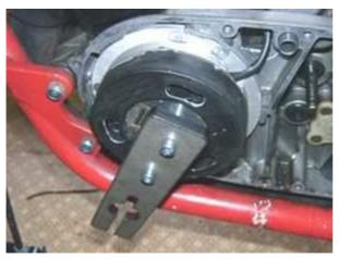
The same tool can be used to pull off the rotor again.
