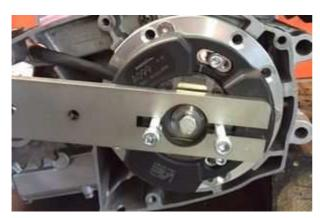
For turning the rotor and stabilizing when fastening, use the enclosed tool as shown.
