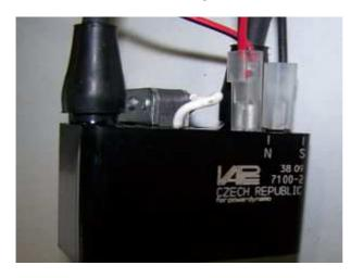
The red/white cable (6.3mm plug) is good for the ignition voltage, the black cable (4.2mm plug) for the pulse. The red/white cable branches - it goes to the kill switch for cut-off the system.
