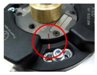
Set the rotor onto the crank in such a way, that the marking on the rotor aligns with the marking on the stator. If there is any change in the crank's position, you have to start again. In that position fasten the rotor carefully. (Please don't forget to use the washer!)
