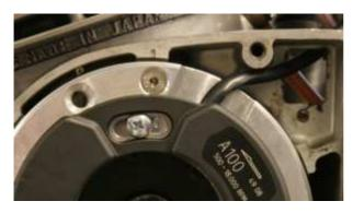
You should set the screws in the center of mounting holes, so you have the possibility for timing correction.
