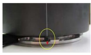
Place the rotor loosely onto the crank and check that it may move freely above the statorbase, check carefully that it clears the heads of the screws holding the inner plate to the adapter. Take the spark plug out and bring the piston into "TDC" (top dead centre) position. As this is difficult to do with the kick lever, using the rotor as a turning knob.
