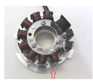
Have a look at the new stator unit. You will find there a near the smallerer black coils a small red marking. This is an ignition marking for timing.
