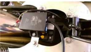
Take during the installation of the advance unit a look at the little blue switching block at the upper narrow side. There are 4 switches for choosing the different advance curves.
