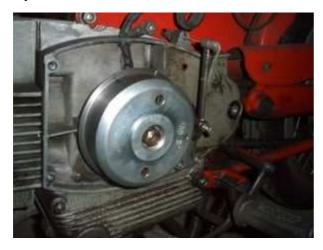
Magnet based generator with integrated fully electronic ignition. Output at 12V/180W DC. Solid state ignition with own power supply from within the system. Completely replaces old magneto system.
