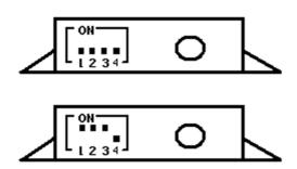
With all switches on OFF (opposite ON) the engine will reach full advance of 38° at 3.000rpm, as it should be.
