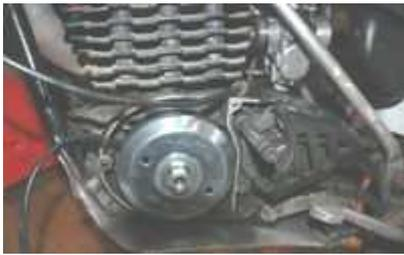
Magnet based solid state ignition. Replaces original Magneto as well as all ignition parts. Does not require changes on crankcase.
