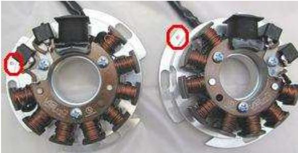
Have a look at the new stator unit. You will find there left from the larger black coil a small red marking. This is an ignition marking for timing.
