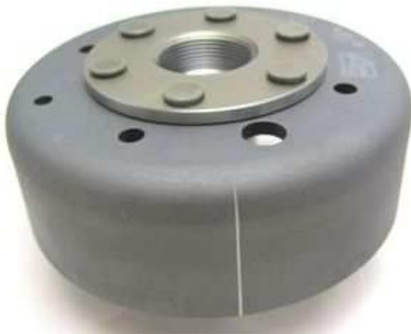
Have a look at the new rotor. You will find on its circumference a lased on (older rotor: pressed in) line. That is an ignition marking too. It is durable, but not well visible, so better highlighten it with some marker pen.
