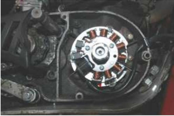
Place the new stator unit onto the engine, same place as the old stator plate had been sitting.
