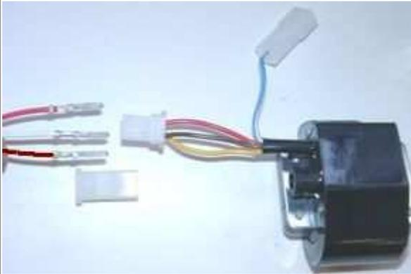
Look for the ignition coil with its female plug and the three wires (red, brown and yellow).
